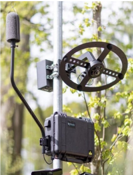
SoundVue™ device that captures and measures noise disturbances]
